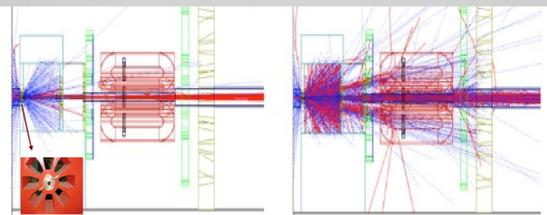
Simulation of beamline backgrounds, with (left) and without (right) the tungsten plug on the upstream collimator. [2]
