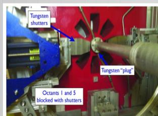
Tungsten shutters blocking octants for a direct measurement of the beamline background component.
