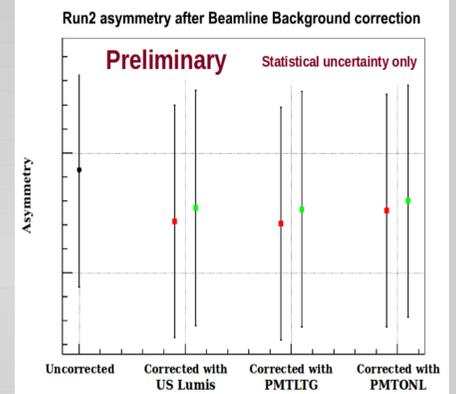
Preliminary agreement between different methods of applying the Beamline Background and the Beam Asymmetries correction. Discrepancy is much smaller than statistical uncertainty.
