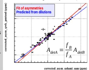
Background asymmetries from different monitors are found to be in excellent agreement and scaling with the monitor’s background signal fraction, as extracted from blocked-octant runs.
