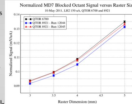
Yield of blocked octants under different raster dimensions and beam conditions. After changes in injector parameters a systematic shift was observed. [2]
